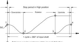
Reference axis for positioning of the input shaft feather
