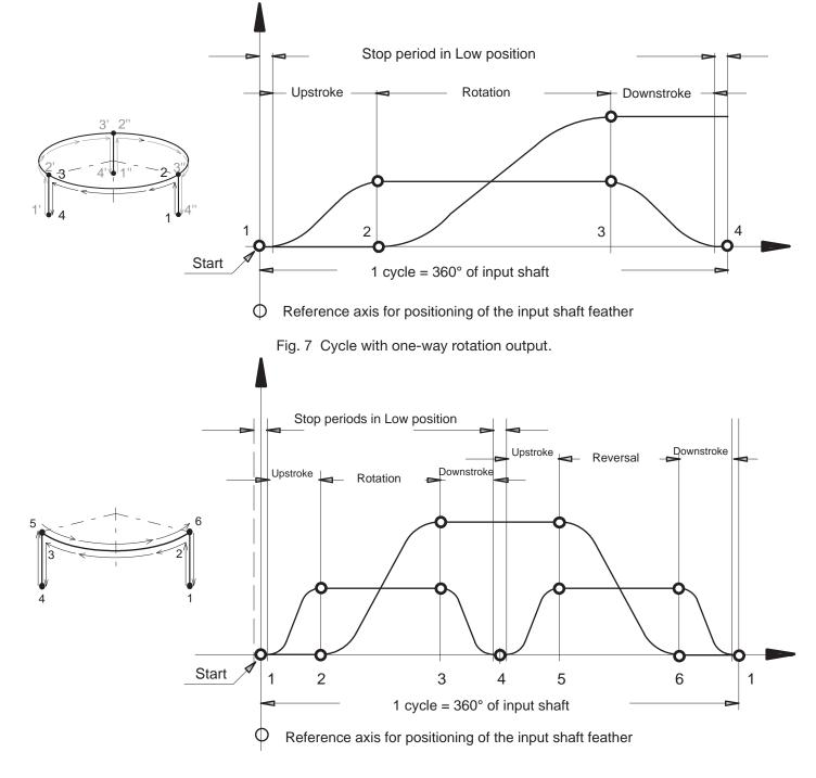
Fig. 8 Cycle with oscillating rotation output.
