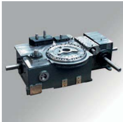
Mechanism with different cams producing seven synchronized intermittent and oscillating movements in output
